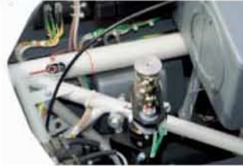
Upper end of special light weight electrical gear drive (left)
