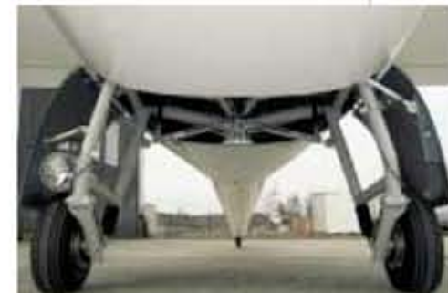
An unconventional gear, to be folded into a minimized fuselage cross section.
