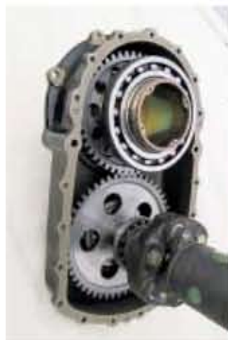
Front gear, opened, for optimized propeller speed and opening for nose cone support
